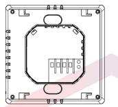
3. Mount with screws the fixed thermostat plate into the electrical connection box.
