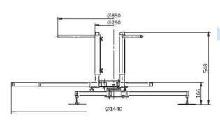
Maximum height of the pipe coil: 660 mm
